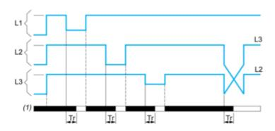
$\mbox{Tr}$ : Response after crossing of threshold (< 300ms) L1, L2, L3: Phases of the supply voltage monitored Alarm status:
